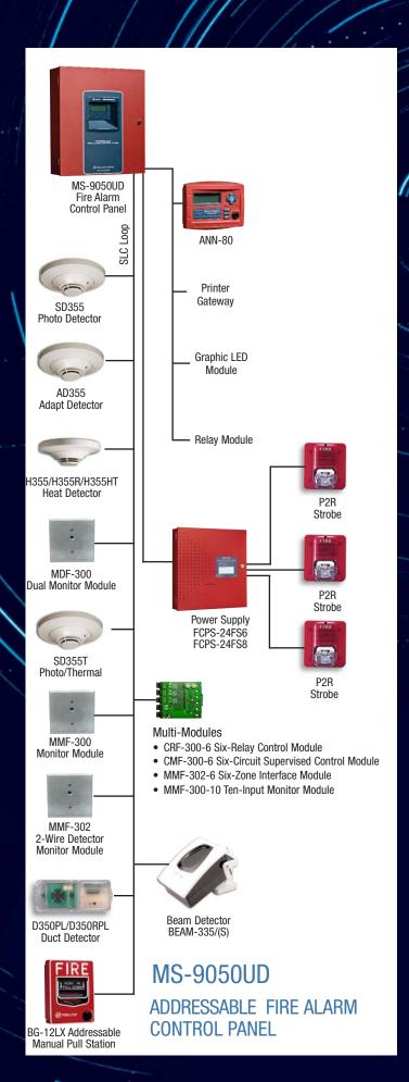
when retrofitting existing devices. The new annunciator bus provides connection for a total of 8 remote devices such as 80-character LCD annunciators for remote display of system status and control of drill, acknowledge and silence functions as well as remote printers, relays and graphic annunciators.
